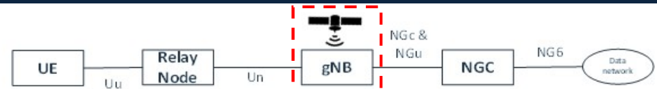
Figure 4.7-4: NTN featuring an access network serving Relay Nodes and based on a satellite/aerial with gNB
