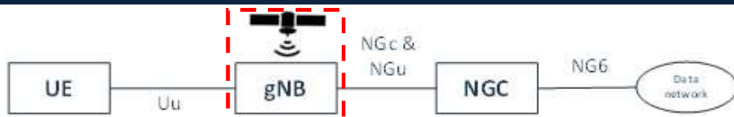
Figure 4.7-2: NTN featuring an access network serving UEs and based on a satellite/aerial with gNB on board
