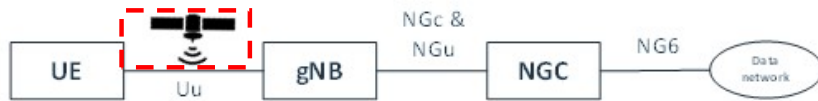
Figure 4.7-1: NTN featuring an access network serving UEs and based on a satellite/aerial with bent pipe payload and gNB on the ground (Satellite hub or gateway level)
