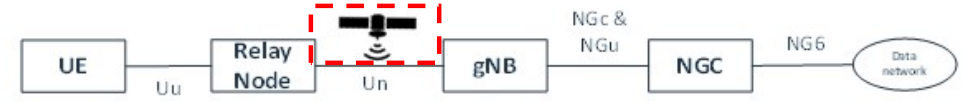
Figure 4.7-3: NTN featuring an access network serving Relay Nodes and based on a satellite/aerial with bent pipe payload
